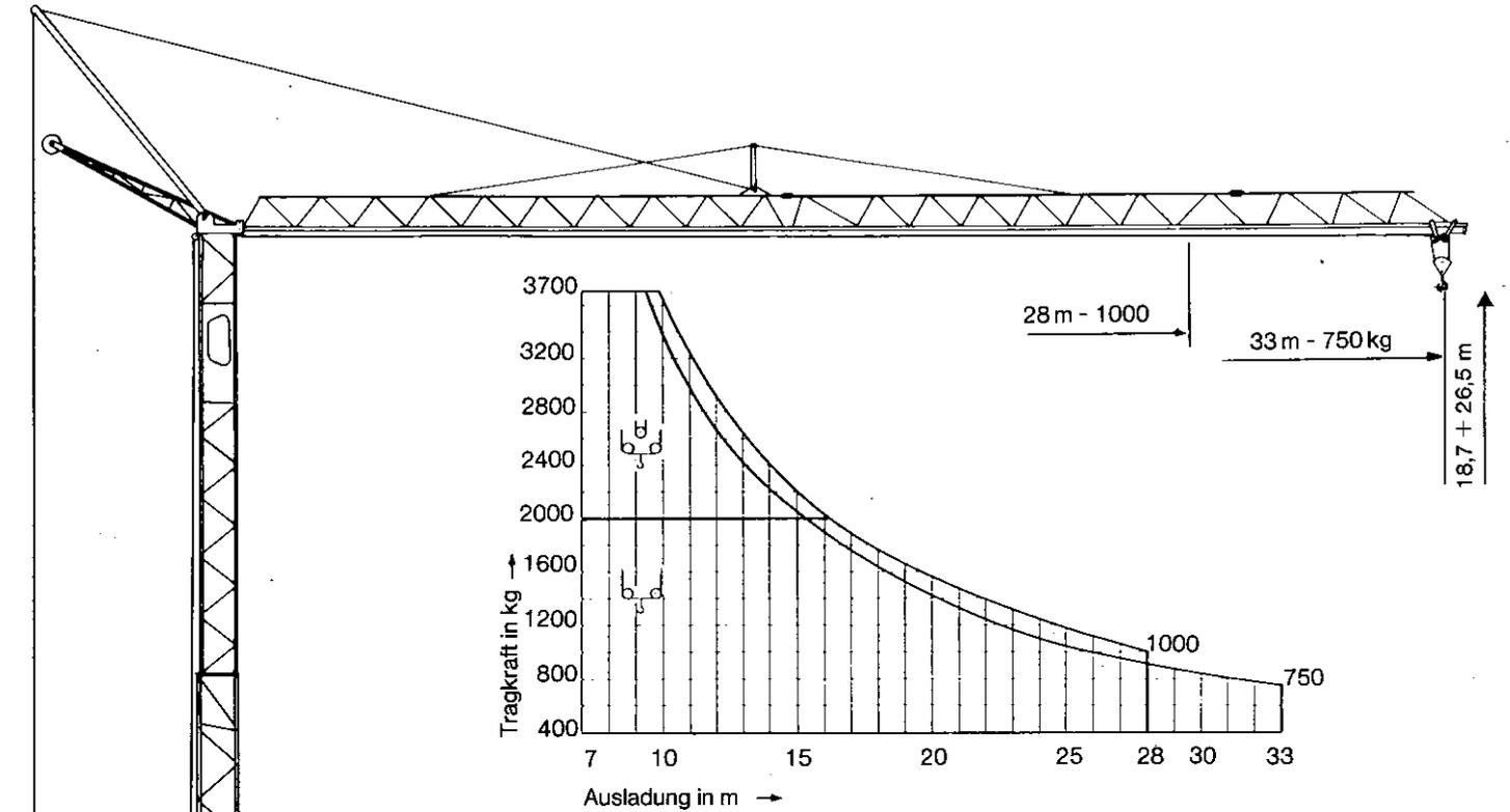
محنى الحمل - Courbes de charges - Loadcurves - Lastkurve
